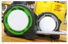
possible to read the tape with the numbers upright regardless of which end of your part you are measuring from. Surprisingly, the tapes also have 1/16" graduations identified with their corresponding numbers – i.e. 7/16" with red number 7, 13/16" with a red 13, etc.!
