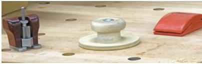
The tool on the left is a custom made router plane which he built and outfitted with a comfortable contoured wooden handle.
