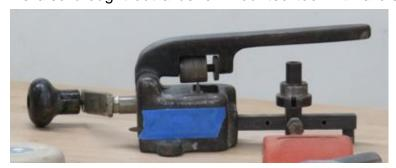
cutting blade. **[Ed Note**: Sure looked a lot like an apple peeling machine to me......::-)] No one could guess what it was, so he finally told us that it was an old manual tool for trimming circular sanding discs!
